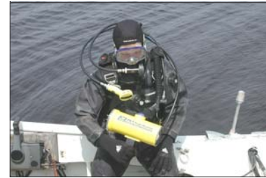
DIVER WITH PINGER RECEIVER PREPARING TO DIVE TO LOCATE PINGER IN WATER.
